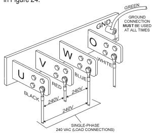
Figure 24. UVWO Terminal Lugs 10/9-240V Connections
